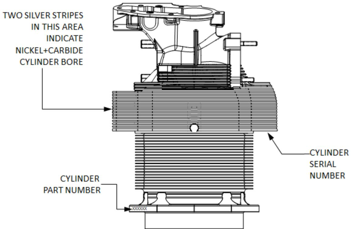
**Figure 1. Cylinder Identification**
