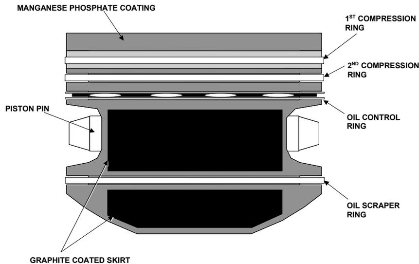
**Figure 4. Piston Ring Installation Order**
